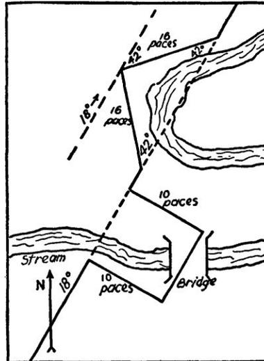
Fig. 10. Two methods of maintaining a compass course around obstacles.
