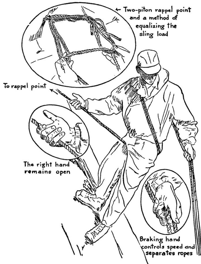
Fig. 19. The body (Dülfer) rappel and a two-piton rappel point.
