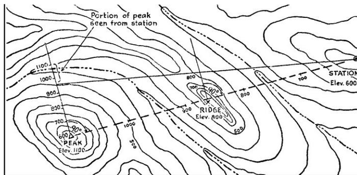
Fig. 11. Method of determining intervisibility.
